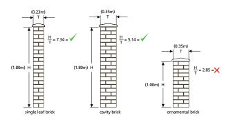
As a general guide, walls with a slenderness ratio (Height/Thickness) of 5:1 or greater may be effectively protected by VibraFon®.
