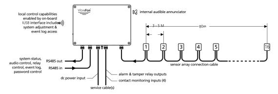
The VibraFon® signal analyser module may be located adjacent to the sensor array deployed on the wall. In such cases, DC power will be required to power the signal analyser and cabling must be provided to route the alarm signals generated by the analyser back to the operator interfaceor annunciation system.
